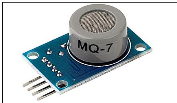
Gambar 2.8 Sensor Gas Karbon Monoksida MQ-7
